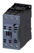
power contactor, AC-3e/AC-3, 41 A, 18.5 kW / 400 V, 3-pole, 110 V AC, 50 Hz, auxiliary contacts: 1 NO + 1 NC, main circuit: screw terminal, control and auxiliary circuit: spring-loaded terminal, size: S2
