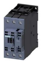
power contactor, AC-3e/AC-3, 41 A, 18.5 kW / 400 V, 3-pole, 220 V AC, 50 Hz / 240 V, 60 Hz, auxiliary contacts: 1 NO + 1 NC, main circuit: screw terminal, control and auxiliary circuit: spring-loaded terminal, size: S2
