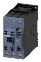
power contactor, AC-3 40 A, 18.5 kW / 400 V 1 NO + 1 NC, 24 V DC with varistor, 3-pole, Size S2, Spring-type terminal Suitable for 2 A PLC outputs
