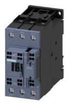
power contactor, AC-3 40 A, 18.5 kW / 400 V 1 NO + 1 NC, AC / DC with varistor, 3-pole, Size S2, Spring-type terminal
