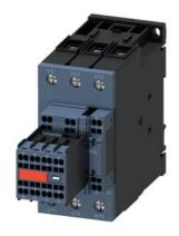
power contactor, AC-3e/AC-3, 41 A, 18.5 kW / 400 V, 3-pole, 20-33 V AC/DC, 50/60 Hz, with integrated varistor, auxiliary contacts: 2 NO + 2 NC, main circuit: screw terminal, control and auxiliary circuit: spring-loaded terminal, size: S2, captive auxiliary switch
