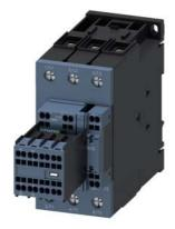
traction contactor, AC-3e/AC-3, 41 A, 18.5 kW / 400 V, 3-pole, 110 V DC, 0.7-1.25  $^{\star}$  Us, electronic drive, with integrated varistor, auxiliary contacts: 2 NO + 2 NC, main circuit: screw terminal, control and auxiliary circuit: spring-loaded terminal, size: S2, removable auxiliary switch
