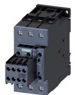
power contactor, AC-3e/AC-3, 51 A, 22 kW / 400 V, 3-pole, 100 V AC, 50 Hz / 100-110 V, 60 Hz, auxiliary contacts: 2 NO + 2 NC, screw terminal, size: S2, removable auxiliary switch
