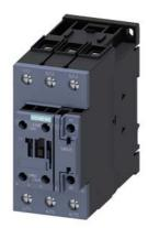
power contactor, AC-3e/AC-3, 51 A, 22 kW / 400 V, 3-pole, 208 V AC, 50/60 Hz, auxiliary contacts: 1 NO + 1 NC, screw terminal
