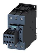
power contactor, AC-3e/AC-3, 51 A, 22 kW / 400 V, 3-pole, 20-33 V AC/DC, 50/60 Hz, with integrated varistor, auxiliary contacts: 2 NO + 2 NC, screw terminal, removable auxiliary switch
