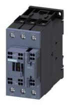
power contactor, AC-3e/AC-3, 51 A, 22 kW / 400 V, 3-pole, 110 V AC, 50 Hz, auxiliary contacts: 1 NO + 1 NC, main circuit: screw terminal, control and auxiliary circuit: spring-loaded terminal, size: S2
