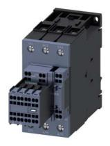
power contactor, AC-3e/AC-3, 51 A, 22 kW / 400 V, 3-pole, 110 V AC, 50 Hz, auxiliary contacts: 2 NO + 2 NC, main circuit: screw terminal, control and auxiliary circuit: spring-loaded terminal, size: S2, removable auxiliary switch
