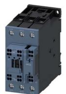
power contactor, AC-3e/AC-3, 51 A, 22 kW / 400 V, 3-pole, 20-33 V AC/DC, 50/60 Hz, with integrated varistor, auxiliary contacts: 1 NO + 1 NC, main circuit: screw terminal, control and auxiliary circuit: spring-loaded terminal, communication-capable
