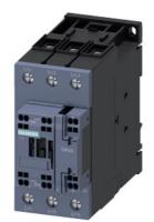
power contactor, AC-3e/AC-3, 51 A, 22 kW / 400 V, 3-pole, 83-155 V AC/DC, 50/60 Hz, with integrated varistor, auxiliary contacts: 1 NO + 1 NC, main circuit: screw terminal, control and auxiliary circuit: spring-loaded terminal, size: S2,
