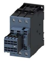
traction contactor, AC-3e/AC-3, 51 A, 22 kW / 400 V, 3-pole, 24 V DC, 0.7-1.25\* Us, electronic drive, with integrated varistor, auxiliary contacts: 2 NO + 2 NC, main circuit: screw terminal, control and auxiliary circuit: spring-loaded terminal, size: S2, removable auxiliary switch
