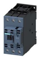
traction contactor, AC-3e/AC-3, 51 A, 22 kW / 400 V, 3-pole, 110 V DC, 0.7-1.25 $^{\star}$  Us, electronic drive, with integrated varistor, auxiliary contacts: 1 NO + 1 NC, main circuit: screw terminal, control and auxiliary circuit: spring-loaded terminal, size: S2
