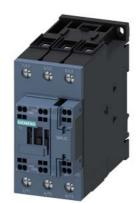
traction contactor, AC-3e/AC-3, 51 A, 22 kW / 400 V, 3-pole, 72 V DC, 0.7-1.25\* Us, electronic drive, with integrated varistor, auxiliary contacts: 1 NO + 1 NC, main circuit: screw terminal, control and auxiliary circuit: spring-loaded terminal, size: S2
