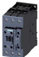
Power contactor, AC-3 65 A, 30 kW / 400 V 1 NO + 1 NC, 230 V AC, 50 Hz 3-pole, size S2 screw terminals
