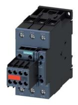
power contactor, AC-3e/AC-3, 65 A, 30 kW / 400 V, 3-pole, 110 V AC, 50 Hz / 120 V, 60 Hz, with plugged-in varistor, auxiliary contacts: 2 NO + 2 NC, screw terminal, size: S2, captive auxiliary switch
