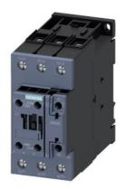
power contactor, AC-3e/AC-3, 65 A, 30 kW / 400 V, 3-pole, 24 V DC, 0.8-1.2\* Us, with integrated varistor, auxiliary contacts: 1 NO + 1 NC, screw terminal, size: S2, upright mounting position, suitable for PLC outputs
