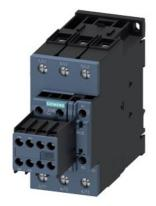
power contactor, AC-3e/AC-3, 65 A, 30 kW / 400 V, 3-pole, 24 V DC, 0.8-  $1.2^{\star}$  Us, with integrated varistor, auxiliary contacts: 2 NO + 2 NC, screw terminal, suitable for PLC outputs
