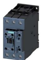
power contactor, AC-3e/AC-3, 65 A, 30 kW / 400 V, 3-pole, 20-33 V AC/DC, 50/60 Hz, with integrated varistor, auxiliary contacts: 1 NO + 1 NC, screw terminal, communication-capable
