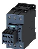
Power contactor, AC-3 65 A, 30 kW / 400 V 2 NO + 2 NC, AC / DC 20-33 V, with varistor 3-pole, size S2 screw terminals
