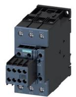
power contactor, AC-3e/AC-3, 65 A, 30 kW / 400 V, 3-pole, 175-280 V AC/DC, 50/60 Hz, with integrated varistor, auxiliary contacts: 2 NO + 2 NC, screw terminal, size: S2, removable auxiliary switch
