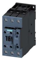
traction contactor, AC-3e/AC-3, 65 A, 30 kW / 400 V, 3-pole, 24 V DC, 0.7-1.25\* Us, electronic drive, with integrated varistor, auxiliary contacts: 1 NO + 1 NC, screw terminal, size: S2
