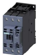
Contactor, AC-3, 30 kW / 400 V, 1 NO + 1 NC, 110 V AC, 50 Hz, 3-pole, Size S2, Spring-type terminal
