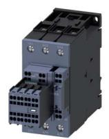
power contactor, AC-3e/AC-3, 65 A, 30 kW / 400 V, 3-pole, 110 V AC, 50 Hz, auxiliary contacts: 2 NO + 2 NC, main circuit: screw terminal, control and auxiliary circuit: spring-loaded terminal, size: S2, removable auxiliary switch
