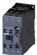
Contactor, AC-3, 30 kW / 400 V, 1 NO + 1 NC, 110 V AC, 50 / 60 Hz, 3-pole, Size S2, Spring-type terminal
