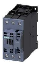
Power contactor, AC-3 65 A, 30 kW / 400 V 1 NO + 1 NC, 220 V AC, 50 Hz 240 V, 60Hz, 3-pole Size S2, Spring-type terminals
