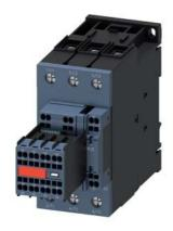
power contactor, AC-3e/AC-3, 65 A, 30 kW / 400 V, 3-pole, 230 V AC, 50/60 Hz, with plugged-in varistor, auxiliary contacts: 2 NO + 2 NC, main circuit: screw terminal, control and auxiliary circuit: spring-loaded terminal, size: S2, captive auxiliary switch
