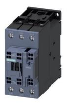
power contactor, AC-3e/AC-3, 65 A, 30 kW / 400 V, 3-pole, 175-280 V AC/DC, 50/60 Hz, with integrated varistor, auxiliary contacts: 1 NO + 1 NC, main circuit: screw terminal, control and auxiliary circuit: spring-loaded terminal, size: S2,
