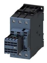
traction contactor, AC-3e/AC-3, 65 A, 30 kW / 400 V, 3-pole, 110 V DC, 0.7-1.25 $^{\star}$  Us, electronic drive, with integrated varistor, auxiliary contacts: 2 NO + 2 NC, main circuit: screw terminal, control and auxiliary circuit: spring-loaded terminal, size: S2, removable auxiliary switch
