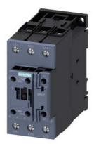
power contactor, AC-3e/AC-3, 80 A, 37 kW / 400 V, 3-pole, 110 V AC, 50 / 60 Hz, auxiliary contacts: 1 NO + 1 NC, screw terminal
