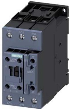
power contactor, AC-3e/AC-3, 80 A, 37 kW / 400 V, 3-pole, 110 V AC, 50 Hz / 120 V, 60 Hz, auxiliary contacts: 1 NO + 1 NC, screw terminal, size: S2, upright mounting position
