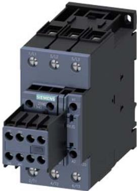
power contactor, AC-3e/AC-3, 80 A, 37 kW / 400 V, 3-pole, 110 V AC, 50 Hz / 120 V, 60 Hz, auxiliary contacts: 2 NO + 2 NC, screw terminal, size: S2, removable auxiliary switch
