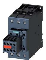
power contactor, AC-3e/AC-3, 80 A, 37 kW / 400 V, 3-pole, 230 V AC, 50/60 Hz, with plugged-in varistor, auxiliary contacts: 2 NO + 2 NC, screw terminal, size: S2, captive auxiliary switch
