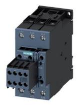
power contactor, AC-3e/AC-3, 80 A, 37 kW / 400 V, 3-pole, 20-33 V AC/DC, 50/60 Hz, with integrated varistor, auxiliary contacts: 2 NO + 2 NC, screw terminal, removable auxiliary switch
