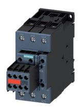
power contactor, AC-3e/AC-3, 80 A, 37 kW / 400 V, 3-pole, 20-33 V AC/DC, 50/60 Hz, with integrated varistor, auxiliary contacts: 2 NO + 2 NC, screw terminal, captive auxiliary switch
