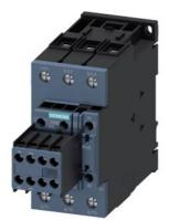
power contactor, AC-3e/AC-3, 80 A, 37 kW / 400 V, 3-pole, 175-280 V AC/DC, 50/60 Hz, with integrated varistor, auxiliary contacts: 2 NO + 2 NC, screw terminal, size: S2, removable auxiliary switch
