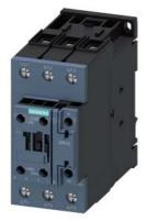
traction contactor, AC-3e/AC-3, 80 A, 37 kW / 400 V, 3-pole, 110 V DC, 0.7-1.25  $^{\star}$  Us, electronic drive, with integrated varistor, auxiliary contacts: 1 NO + 1 NC, screw terminal, size: S2
