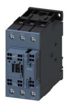
power contactor, AC-3e/AC-3, 80 A, 37 kW / 400 V, 3-pole, 20-33 V AC/DC, 50/60 Hz, with integrated varistor, auxiliary contacts: 1 NO + 1 NC, main circuit: screw terminal, control and auxiliary circuit: spring-loaded terminal, communication-capable
