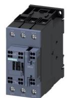
power contactor, AC-3e/AC-3, 80 A, 37 kW / 400 V, 3-pole, 175-280 V AC/DC, 50/60 Hz, with integrated varistor, auxiliary contacts: 1 NO + 1 NC, main circuit: screw terminal, control and auxiliary circuit: spring-loaded terminal
