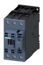
traction contactor, AC-3e/AC-3, 80 A, 37 kW / 400 V, 3-pole, 24 V DC, 0.7-1.25\* Us, electronic drive, with integrated varistor, auxiliary contacts: 1 NO + 1 NC, main circuit: screw terminal, control and auxiliary circuit: spring-loaded terminal, size: S2
