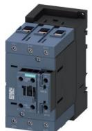
power contactor, AC-3e/AC-3, 80 A, 37 kW / 400 V, 3-pole, 175-280 V AC/DC, 50/60 Hz, with integrated varistor, auxiliary contacts: 1 NO + 1 NC, screw terminal
