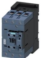
traction contactor, AC-3e/AC-3, 80 A, 37 kW / 400 V, 3-pole, 110 V DC, 0.7-1.25\* Us, electronic drive, with integrated varistor, auxiliary contacts: 1 NO + 1 NC, screw terminal
