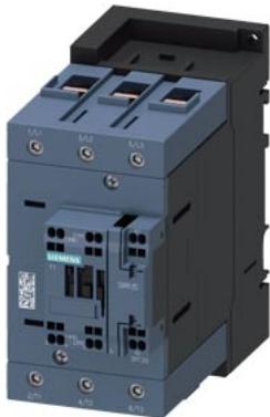
traction contactor, AC-3e/AC-3, 80 A, 37 kW / 400 V, 3-pole, 24 V DC, 0.7-1.25\* Us, electronic drive, with integrated varistor, auxiliary contacts: 1 NO + 1 NC, main circuit: screw terminal, control and auxiliary circuit: spring-loaded terminal
