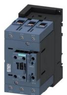
power contactor, AC-3e/AC-3, 95 A, 45 kW / 400 V, 3-pole, 24 V DC, 0.8-  $1.2^*$  Us, with integrated varistor, auxiliary contacts: 1 NO + 1 NC, screw terminal, suitable for PLC outputs
