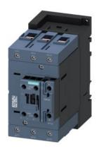
power contactor, AC-3e/AC-3, 95 A, 45 kW / 400 V, 3-pole, 24 V DC, 0.8-1.2\* Us, with integrated varistor, auxiliary contacts: 1 NO + 1 NC, screw terminal, suitable for PLC outputs, upright mounting position
