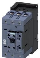
power contactor, AC-3e/AC-3, 95 A, 45 kW / 400 V, 3-pole, 20-33 V AC/DC, 50/60 Hz, with integrated varistor, auxiliary contacts: 1 NO + 1 NC, screw terminal, communication-capable
