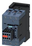
power contactor, AC-3e/AC-3, 95 A, 45 kW / 400 V, 3-pole, 20-33 V AC/DC, 50/60 Hz, with integrated varistor, auxiliary contacts: 2 NO + 2 NC, screw terminal, captive auxiliary switch
