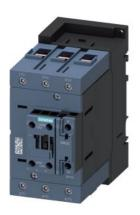
traction contactor, AC-3e/AC-3, 95 A, 45 kW / 400 V, 3-pole, 110 V DC, 0.7-1.25\* Us, electronic drive, with integrated varistor, auxiliary contacts: 1 NO + 1 NC, screw terminal
